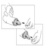
2 - Load the gun with a pin and ferrule
